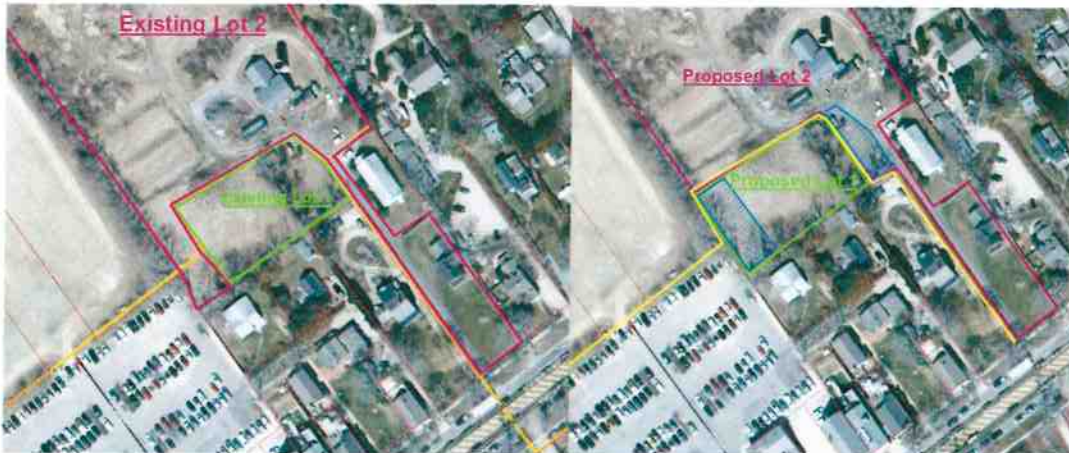
Rough sketches showing approximate location of the existing lots (purple and green), areas to be transferred between lots (blue), and zoning boundary (yellow) and proposed lots and zoning boundary
